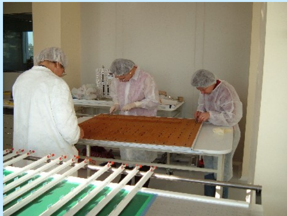
Final check of the Honeycomb Panel
