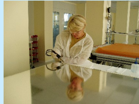
Dispersing the glue between Frame and Radiator
