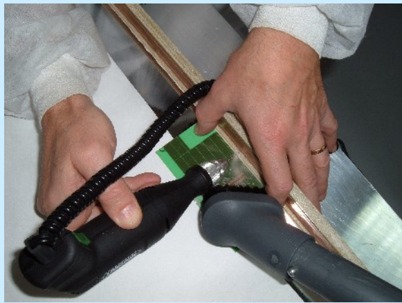
Drilling the hole for the Drift HV cable
