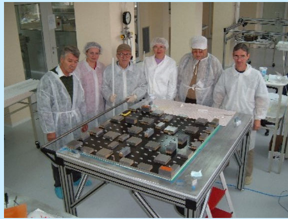
Distributed weight on the Honeycomb Panel during polymerisation
