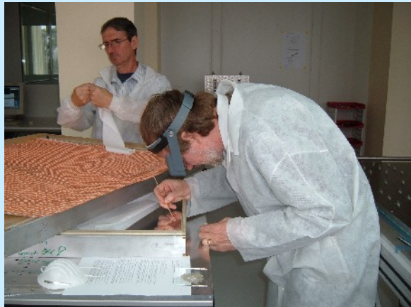
Drift HV connection on the Radiator
