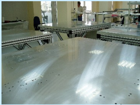
2 pairs of Glueing & Vacuum Tables installed
